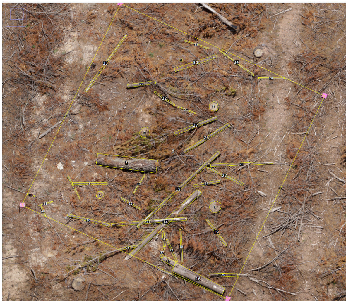
Figure 3. Imagery and annotation data for plot number 4 of 9: photomosaic layer with overlaid plot boundaries ( 10 \times 10 m quadrat) and digitally annotated locations/boundaries of all coarse woody debris with diameter greater than 2.5 cm.
