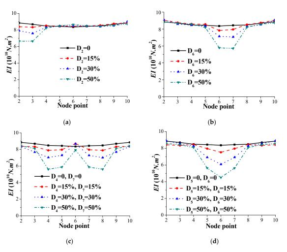
**Figure 17.** Estimated element bending stiffness *EI* of bridge for Case 2: (**a**) Scenario A; (**b**) Scenario B; (**c**) Scenario C; (**d**) Scenario D.
