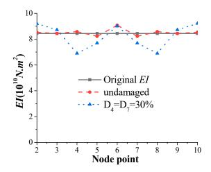
**Figure 23.** Identified element bending stiffness EI from the combined effect analysis: undamaged scenario & Scenario C,  $D_4 = 30\%$  and  $D_7 = 30\%$ .
