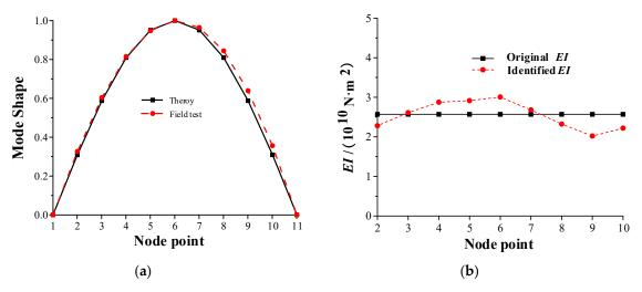
Figure 36. Identified results of the 3rd span for field test: (a) Mode shape; (b) Bending stiffness EI.
