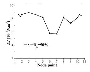
Figure 24. Estimated element bending stiffness El with refined finite element close to the boundary
