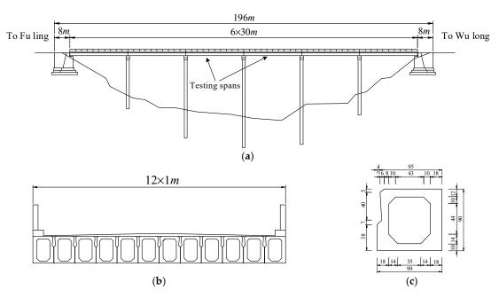
Figure 27. Testingbridge: (a) Bridge elevation; (b) Bridge cross-section; (c) Girder cross-section.
