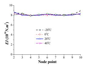
Figure 21. Estimated element bending stiffness El from measurements at different ambient temperature.
