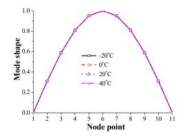
Figure 20. 1st vibration mode shape of the intact bridge at different ambient temperatures.
