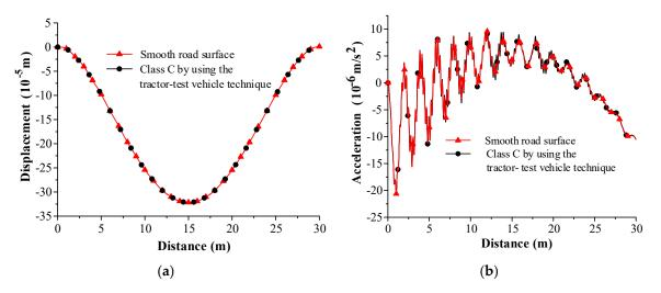
**Figure 6.** Comparison of a single vehicle-bridge system (without tractor and roughness) and tractor-test vehicle technique (Class C road surface roughness): (**a**) Displacement; (**b**) Acceleration.
