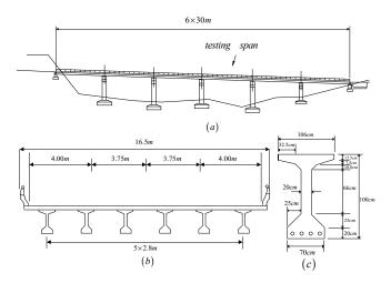
Figure 4. Bridge for simulation: (a) Elevation; (b) Cross-section; (c) Girder cross-section.
