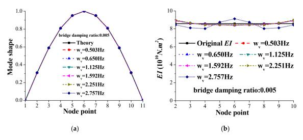
**Figure 10.** Identified results for different vehicle frequencies with bridge damping ratio  $\xi_n = 0.005$ : (a) Mode shape; (b) Element bending stiffness *EI*.
