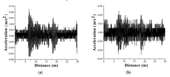
Figure 33. The acceleration response of: (a) big test vehicle; (b) small test vehicle.
