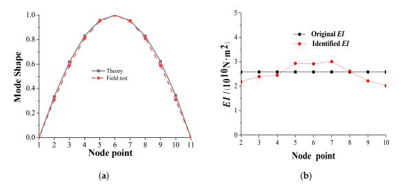
Figure 35. Identified results of the 4th span for field test: (a) Mode shape; (b) Bending stiffness EI.
