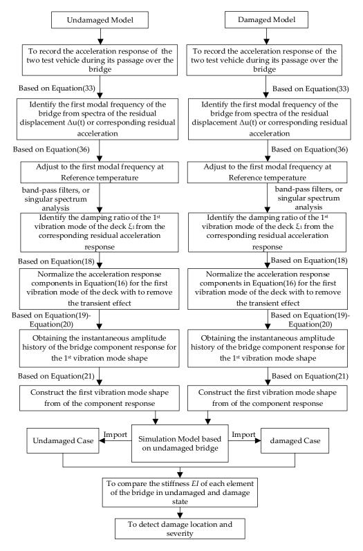
Figure 3. Flow chart of damage identification by using the tractor-test vehicle technique.
