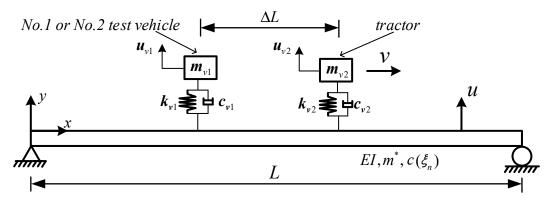
Figure 1. Spring mass moving over a bridge.
