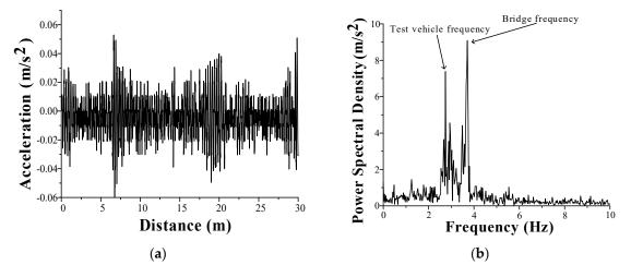
Figure 34. (a) Time history and; (b) Power spectral density of the residual acceleration signals.
