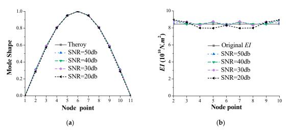
**Figure 14.** Identified results for different signal-to-noise ratio: (**a**) Mode shape; (**b**) Element bending stiffness *EI*.
