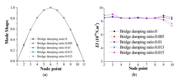
**Figure 13.** Contrast diagram of different damping ratios of the bridge with undamaged conditions for Class C of road surface roughness: (a) Mode shape; (b) Element bending stiffness *EI*.
