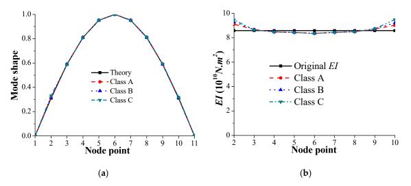
**Figure 12.** Identified resultsfor three classes of road surface roughness with bridge damping ratio  $\xi_n = 0.01$ : (a) Mode shape; (b) Element bending stiffness *EI*.
