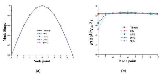
**Figure 25.** Identified results for different left bearing stiffness reduction: (**a**) Mode shape and; (**b**) element bending stiffness *EI*.
