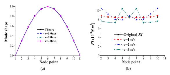
**Figure 7.** Identified resultsfor different vehicle speeds: (**a**) Mode shape and; (**b**) Element bending stiffness *EI*.
