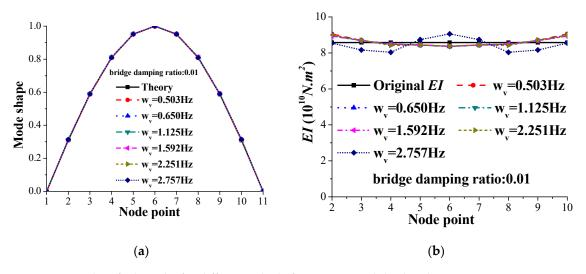
**Figure 11.** Identified results for different vehicle frequencies with bridge damping ratio  $\xi_n = 0.01$ : (a) Mode shape; (b) Element bending stiffness *EI*.
