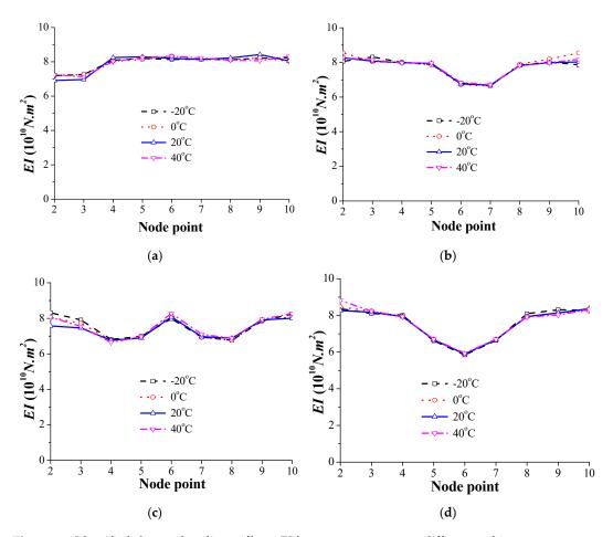
**Figure 22.** Identified element bending stiffness *EI* from measurements at different ambient temperatures: (a) Scenario A,  $D_2 = 30\%$ ; (b) Scenario B,  $D_6 = 30\%$ ; (c) Scenario C,  $D_4 = 30\%$  and  $D_7 = 30\%$ ; (d) Scenario D,  $D_5 = 30\%$  and  $D_6 = 30\%$ .
