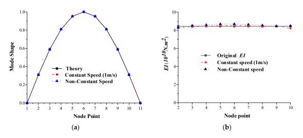
**Figure 9.** Identified results for non-constant speed: (**a**) Mode shape and; (**b**) Element bending stiffness *EI*.
