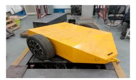
Figure 31. The single-axletest vehicle is tested on a shaking table.
