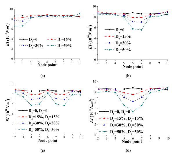
**Figure 18.** Estimated element bending stiffness *EI* of the bridge for Case 3 with Class C road surface roughness: (**a**) Scenario A; (**b**) Scenario B; (**c**) Scenario C; (**d**) Scenario D.
