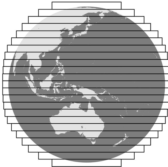
**Figure 2.** Schematic of HIMAWARI-8/Advanced HIMAWARI Imager (AHI) scanning. Each horizontal band represents a scanning swath. Scanning direction is west to east.
