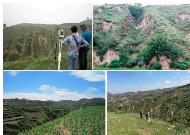
Figure 3. Field survey. Bank gully heads were measured by GNSS and total station in the study area.
