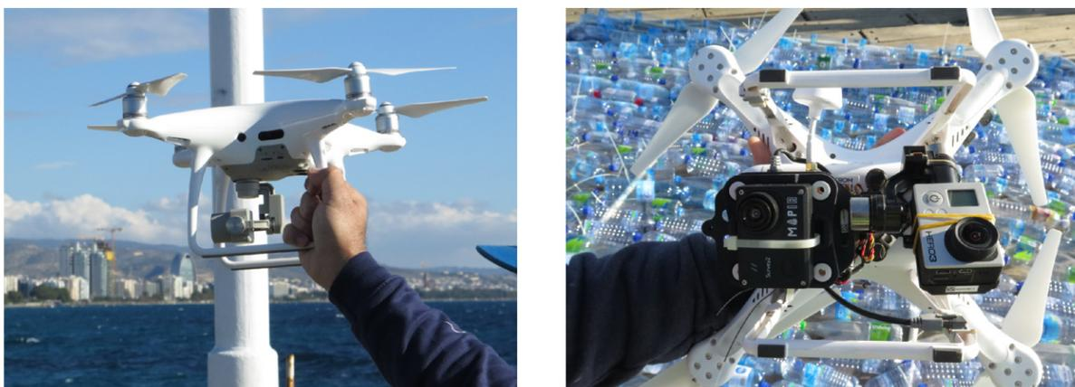
**Figure 4. Left:** Phantom 4 Pro with RGB integrated 20MP camera. Kyriacos Themistocleous.
