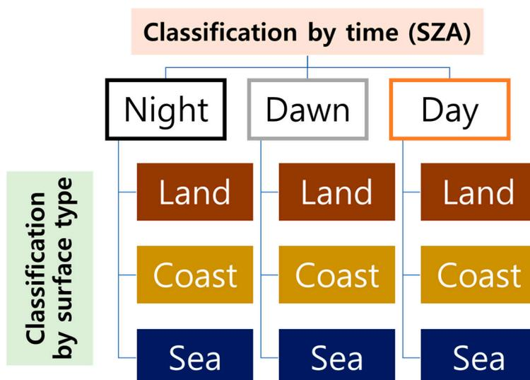
**Figure 3.** Differentiation of fog detection algorithms, according to the solar zenith angle (SZA) and geographic location.
