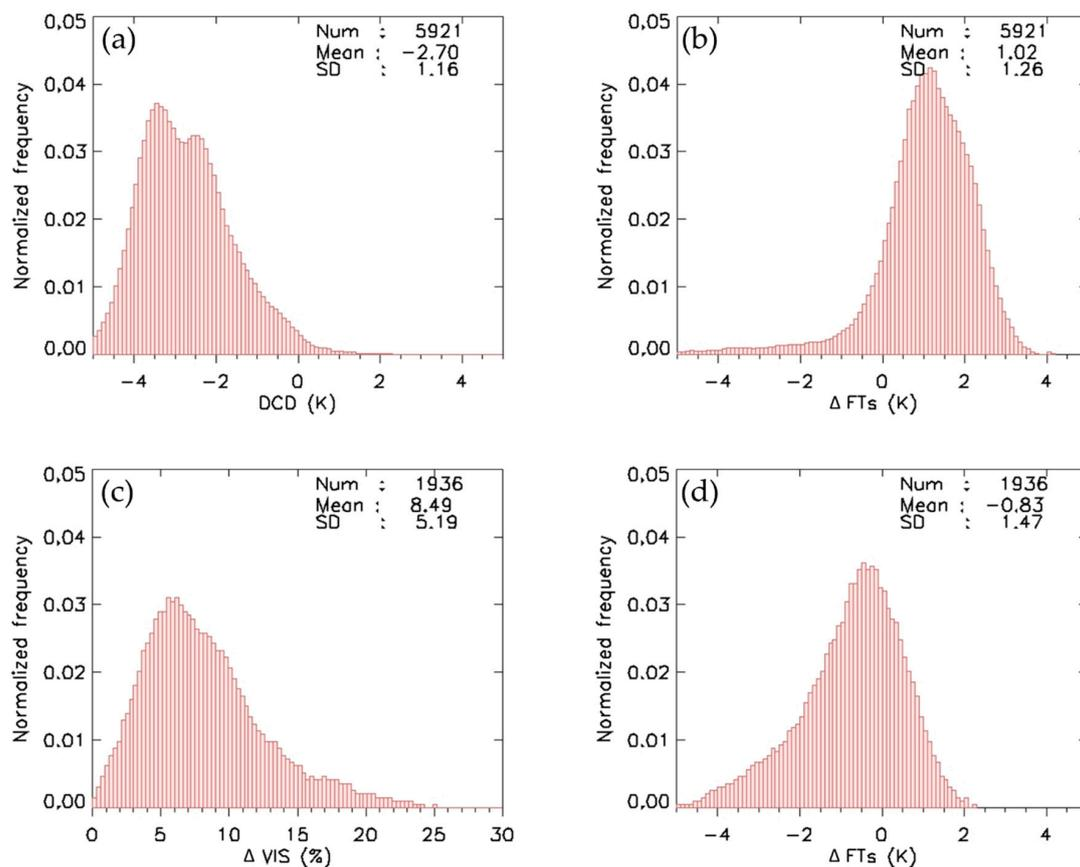
**Figure 5.** Frequency distribution of the optical/textural properties of fog pixels in the training cases at nighttime (a,b) and daytime (c,d). (a) Dual Channel Difference (DCD), (b,d) Difference between the BT of the fog top and surface temperature ( $\Delta$ FTs), and (c) Difference between the reflectance of  $0.64 \mu\text{m}$  (VIS0.6) and Vis\_Comp ( $\Delta$ VIS).
