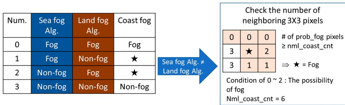
**Figure 4.** Conceptual diagram for the spatial blending method. The part marked with a star indicates a case where the results of the sea fog algorithm and the land fog algorithm are different from each other.
