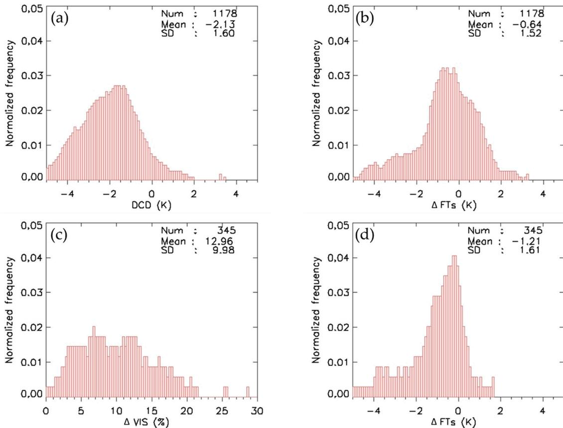
**Figure 6.** Frequency distribution of the optical/textural properties of fog pixels in the training cases at nighttime (a,b) and daytime (c,d) on the coast. (a) DCD, (b,d)  $\Delta FTs$ , and (c)  $\Delta VIS$ .
