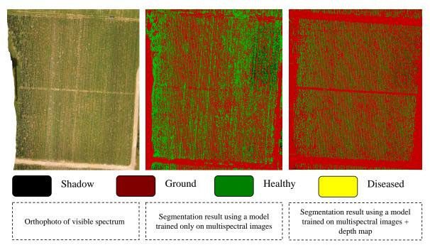
**Figure 7.** Difference between a SegNet model trained only on multispectral data and the same trained on multispectral data combined with depth map information. The presented example is on an orthophoto of a healthy parcel with a green ground.
