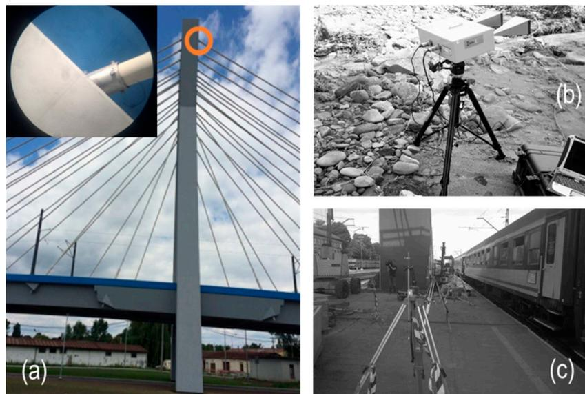
**Figure 5.** Pictures showing the used techniques and measuring devices: (a) total station; (b) IBIS radar; (c) leveling and gauges.
