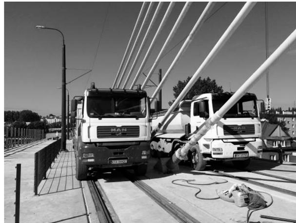
**Figure 3.** A picture showing static load test.
