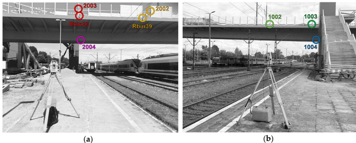
**Figure 6.** A view of the flyover span under study from the (a) northern and (b) southern position together with the marking of the location of the observed points.
