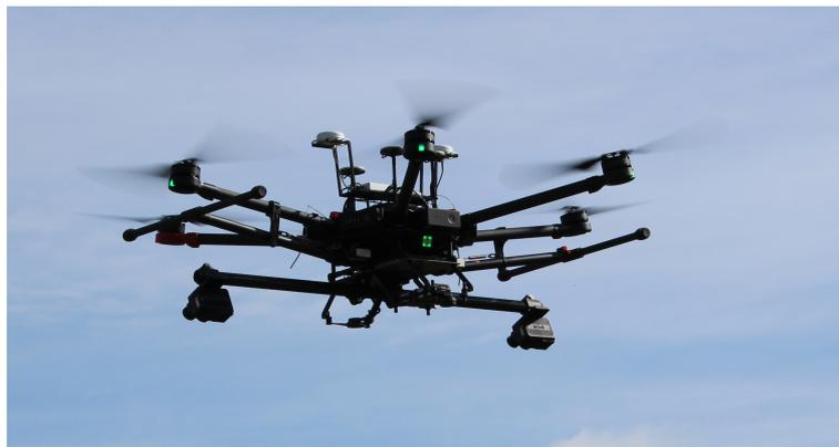
**Figure 1.** Stereovision system with two multimodal cameras fixed on an M600 DJI unmanned aerial vehicle (UAV).
