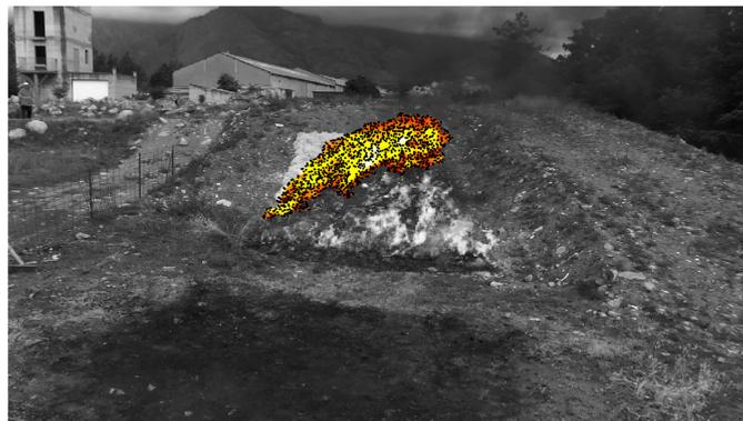
**Figure 29.** Detected frontal fire area and matched points.
