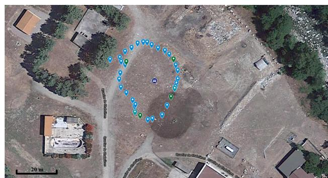
**Figure 17.** Drone and car positions registered by global positioning system (GPS) sensors. The light blue icons represent the positions of the drone during the test, the green icons represent the positions of the drone when the picture was captured, and the dark blue icon represents the position of the car.
