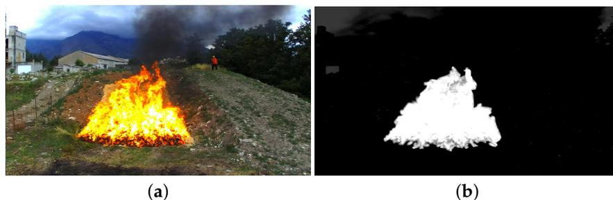
**Figure 3.** Example of images acquired simultaneously in the (a) visible and (b) long wavelength infrared spectra.
