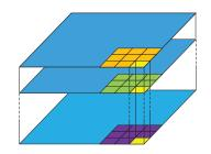
Figure 6. Depthwise separable convolution.
