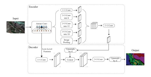
Figure 5. Structure diagram of DeepLab V3+.
