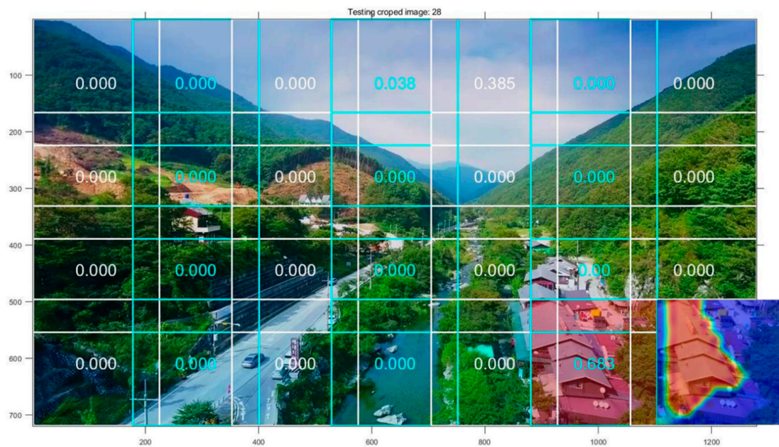
Figure 11. Example of model application with softmax result for non-wildfire (with error).
