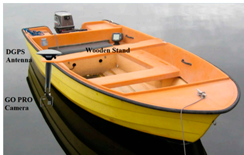
Figure 4. An illustration of the towed camera and the differential global positioning system (DGPS) positions on the motorboat.
