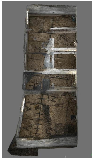
Figure 7. Dense point cloud obtained by photogrammetric survey.
