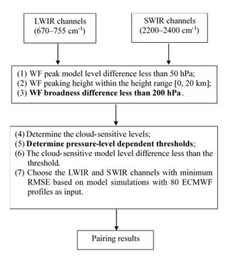
**Figure 5.** Flow chart summarizing three major steps in the HIRAS LWIR/SWIR pairing procedure. Modifications added in this study to original method are indicated in bold.
