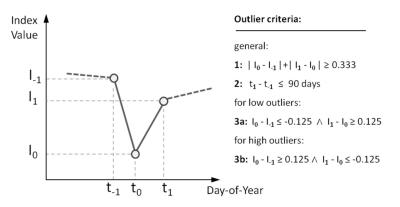
Figure 2. Schematic graph to illustrate criteria for outlier filtering (of I<sub>0</sub>).
