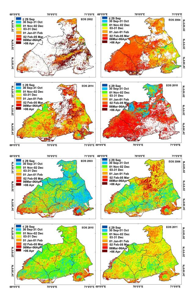
Figure S1. End of Season (EOS) for four dry years (2002, 2004, 2014, 2018), and four wet years (2003, 2006, 2010, 2011), derived from TIMESAT using NDVI thresholds of 35% for SOS and 10% for EOS from base of seasonal NDVI curve. EOS is incorrectly shown as March-April for most areas in dry years and for many areas in wet years, whereas the growing season normally ends in October to November of the previous year.
