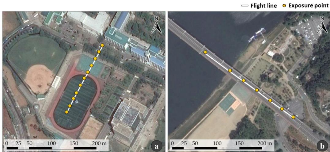
**Figure 1.** Flight lines and exposure points for the two image strips: (a) the flight plan for Dataset-1A and (b) the flight plan for Dataset-1B. These figures were formulated by editing Figure 5; Figure 15 from the work of Kim et al. [18].
