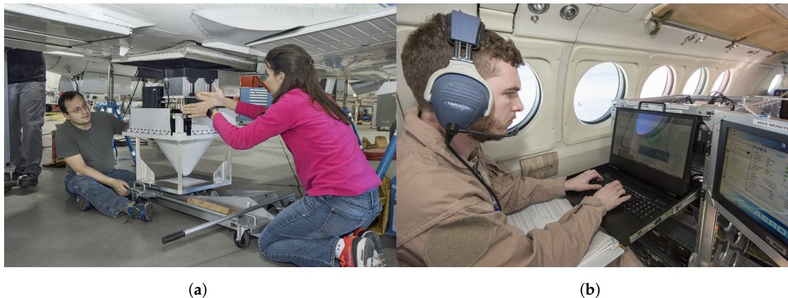
Figure 8. (a) DopplerScatt engineers Raquel Monje and Fabien Nicaise install the instrument into the NASA King Air B200 nadir-looking port. Photo Credit: Ken Ulbrich, NASA AFRC (b) DopplerScatt operator Alex Wineteer, in flight, monitors instrument health and incoming backscatter data, seated in front of the instrumentation rack. Photo Credit: Carla Thomas, NASA AFRC
