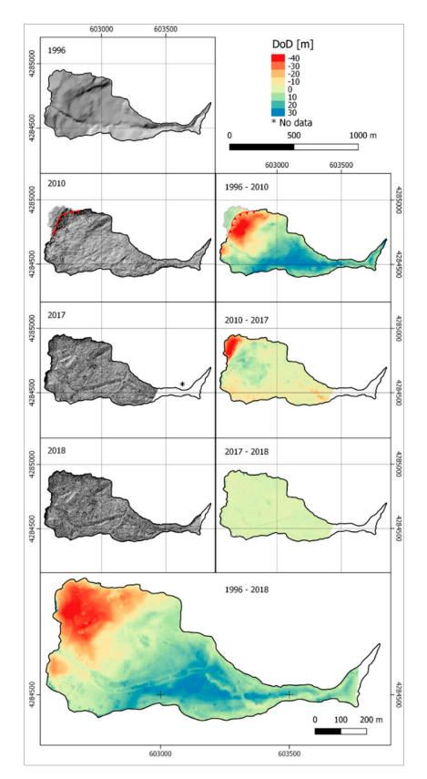
**Figure 7.** Hillshades (left) and DEM of differences (DoDs) (right) of the landslide (RS: UTM WGS84—Zone 33N; EPSG code 32633). The red line in the 2010 hillshade and in the 1996–2010 DoD represent the landslide scarp of 15 February 2010.
