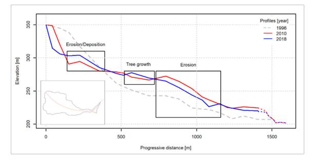
**Figure 11.** Cross section comparison depicting landslide evolution, the dotted lines represents the hypothetical profile outside the landslide border connecting with the undisturbed one.
