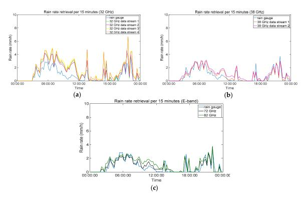
**Figure 8.** Average rain rate per 15 min derived from the signal link compared with the rain gauge measurement on 7 June 2017: (a) 32 GHz link; (b) 38 GHz link; (c) E-band link.
