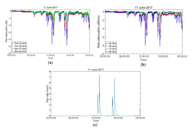
**Figure 5.** (**a**) Received signal variation of the test links on June 11, 2017. (**b**) received signal variation of the test links averaged over 1 km distance. (**c**) rain rate monitored by a rain gauge.
