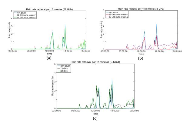
**Figure 9.** Average rain rate per 15 min derived from the signal link compared with the rain gauge measurement on 11 June 2017: (**a**) 32 GHz link; (**b**) 38 GHz link; (**c**) E-band link.
