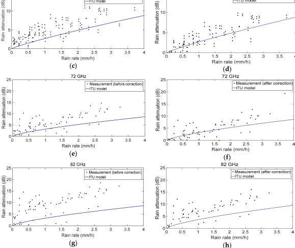
Figure 7. Rain attenuation statistics from the measurement before correction and after correction in comparison with the calculated rain attenuation, using the ITU model from Equation (9) for different frequencies: (a,b) 32 GHz; (c,d) 38 GHz; (e,f) 72 GHz; (g,h) 82 GHz.
