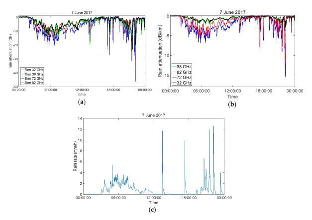
**Figure 4.** (**a**) Received signal variation of the test links on June 7, 2017; (**b**) received signal variation of the test links averaged over 1 km distance; (**c**) rain rate monitored by a rain gauge.
