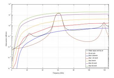
**Figure 1.** Frequency-dependent attenuation of electromagnetic radiation in standard atmosphere (barometric pressure 1013 mbar, temperature 15 °C, water vapor density of 7.5 g/m<sup>3</sup>) and rain attenuation in dB/km at various rainfall rates.
