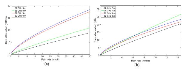
**Figure 2.** The theoretical rain-induced signal attenuation for various rain rates at different frequencies: (a) per kilometer; (b) over a 7-km long 32 GHz 2 × 2 line-of-sight multiple-input multiple-output (LOS-MIMO) link, a 7-km long single-input single-output (SISO) 38 GHz link, a 3-km long 72 GHz link, and a 3-km long 82 GHz test link using our measurement scenario.
