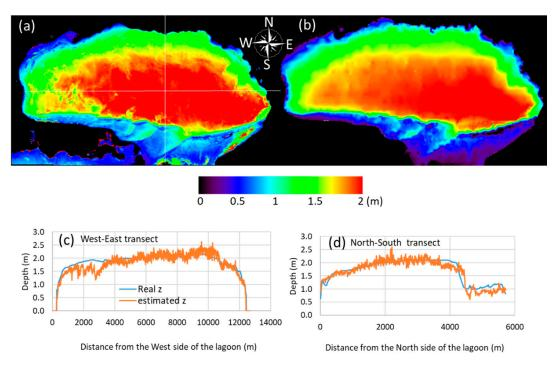
**Figure 5.** (a) Retrieved water depth from the simulated BIODIVERSITY datasets; (b) water depth measured in situ using a sounder provided by RNC institute; (c) west–east distribution of water depth along a transect at 43.54° latitude, (d) north–south water depth along a transect at 4.57° longitude. The two transects are identified on Figure 5a by white lines.
