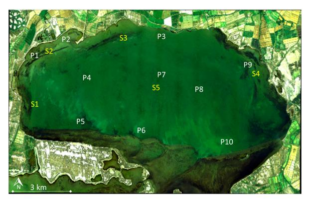
**Figure 2.** Red-green-blue (RGB) mosaic measured by HYSPEX airborne instrument. The positions of the in situ sampling stations (stations noted P) and underwater bottom image acquisitions using an in situ camera (stations noted S) are reported.
