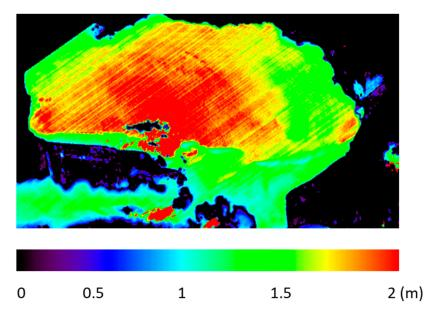
**Figure 9.** Inversion of DESIS data to retrieve water depth using Lee's method. The DESIS satellite image was acquired on 1 February 2020.
