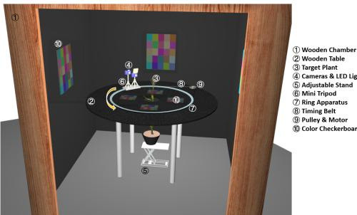
② Wooden Table ③ Target Plant ④ Cameras & LED Light (5) Adjustable Stand 6 Mini Tripod ⑦ Ring Apparatus ⑧ Timing Belt (9) Pulley & Motor 1 Color Checkerboard
