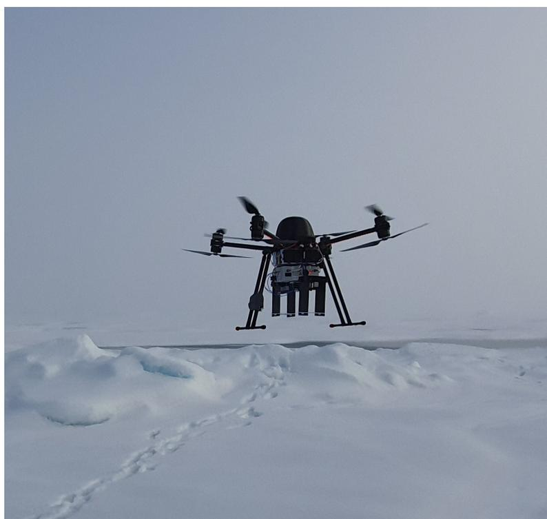
**Figure 1.** UWibaSS mounted under the UAV Cryocopter FOX during flight.
