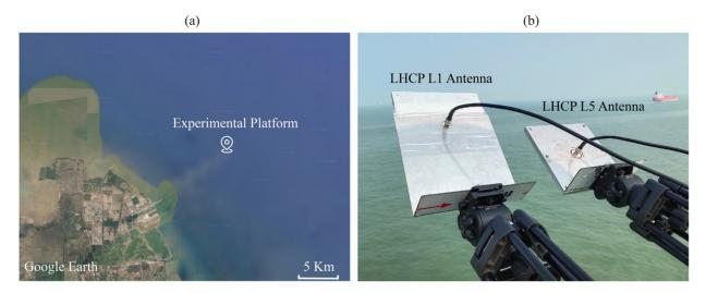
**Figure 4.** GNSS-R experiment setup at Dongying, China. (a) Aerial image (Google Earth) of the experimental site. (b) Photograph of the side-looking LHCP antennas, including the GPS L1 antenna and GPS L5 antenna.
