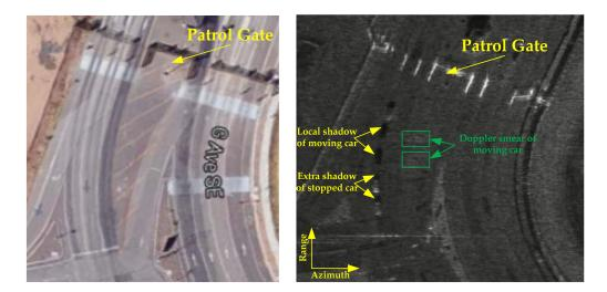
Figure 9. Shadow features of ground moving car shown in real ViSAR image.
