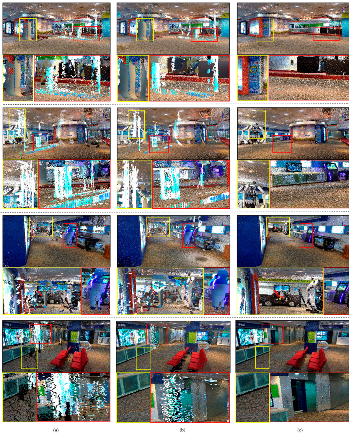
Figure 17. Comparison of the reflective noise results. (a) is the original point cloud image, (b) is the result after processing by FARO SENCE filter, and (c) is the result obtained by our method.
