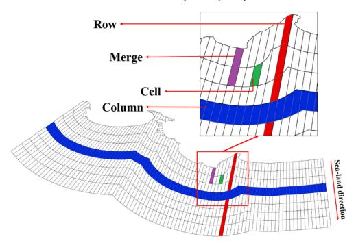
Figure 2. Schematic diagram of the grid division.
