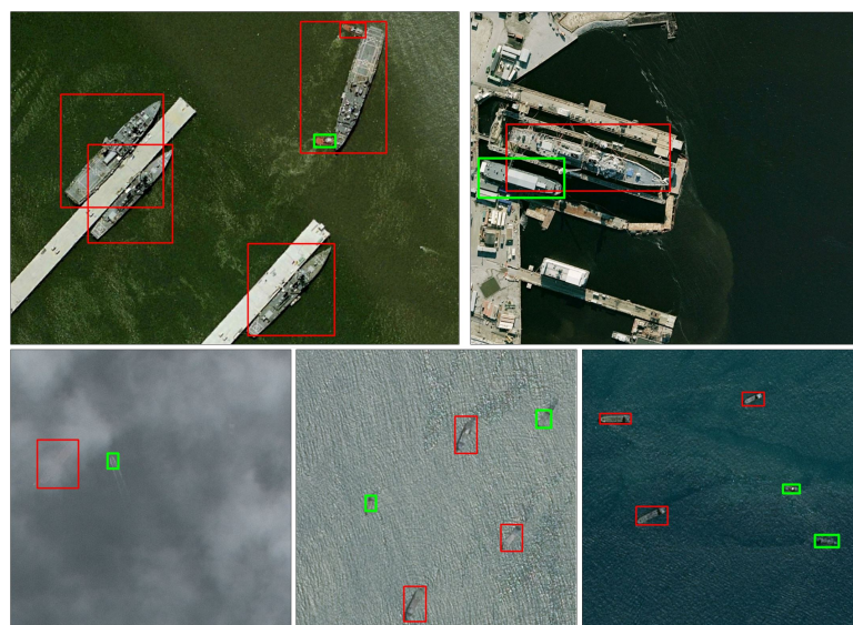
Figure 13. Some failed cases of the proposed method. The missed detections are marked by green boxes.
