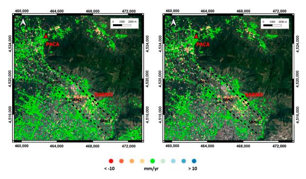
**Figure 11.** Mean displacement rate map for ENVISAT images (2003–2010 period): (**a**) ascending and (**b**) descending. Red triangle indicates location of GNSS Palma Campania (PACA).
