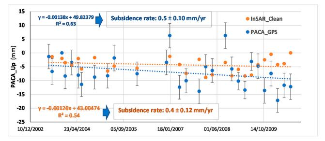
Figure 12. Comparison of GNSS and DInSAR time series (vertical component) collected in Palma Campania with the aim of validating the DInSAR data.
