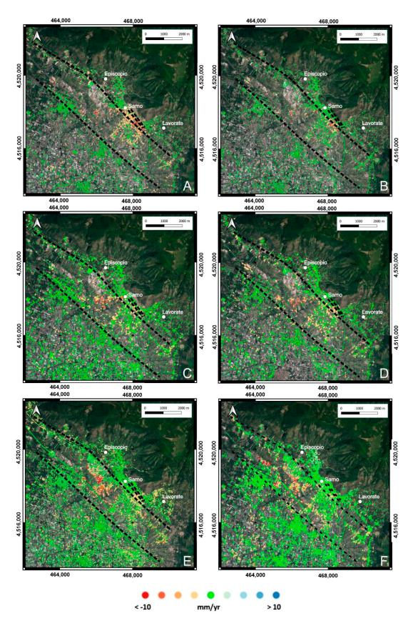
**Figure 10.** Mean displacement rate maps for: ERS1/2, (**A**) ascending and (**B**) descending; ENVISAT: (**C**) ascending and (**D**) descending; (**E**) Cosmo-SkyMed images in descending orbit; and (**F**) SENTINEL-1 images in descending orbit (2016–2020 time span). Dashed black lines indicate faults inferred by geomorphological and stratigraphic analysis (see Figure 4).
