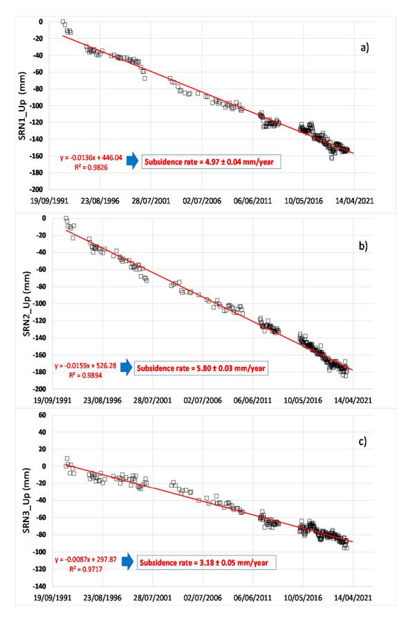
**Figure 13.** Time series of the DInSAR data (up component) used to characterise the vertical displacements within the Sarno basin (**a–c**). Refer to Figure 11 to locate the selected points.
