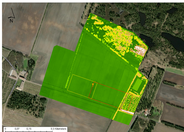
Figure 1. Illustration of the agricultural area (56.037644° N, 9.159383° E) surveyed by the Unmanned aerial vehicle-Light detection and ranging (UAV-LiDAR) system (30.68 ha), and the two subscenes with a range of roughness element densities: Plot 1 with more homogeneous heights corresponding to the wind regime 190° to 347° (yellow, left rectangle), and Plot 2 with more heterogeneous heights corresponding to the wind regime spanning from 90° to 190° (red, right rectangle). The orange label indicates the location of the Eddy covariance tower.
