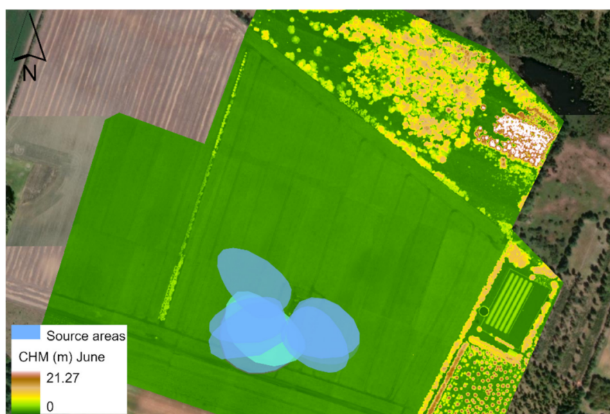
Figure 7. Canopy height model of the agricultural site as obtained by the UAV-LiDAR survey in June. The ellipsoid shapes indicate the probable surface areas contributing to turbulent flux measurements imposing the respective prevailing meteorological conditions.
