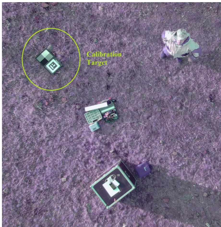
Figure 5. MAPIR calibration target.
