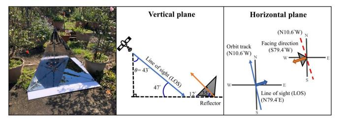
**Figure 2.** Geometry of the corner reflector designed for the ascending orbital geometry of the Sentinel-1 satellite, which was set up at the upper part of the Huafan University campus. The elevation of the corner reflector is 12 degrees and faces S79.4°W, which can effectively reflect the signal from the SAR sensor with a maximum response.
