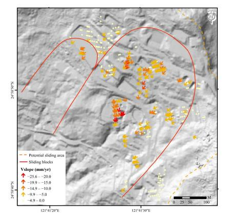
**Figure 5.** The projection of both ascending and descending LOS velocities along the downslope direction. The slow-moving phenomenon was significant, and the maximum displacement velocity along the downslope direction was approximately 25 mm/yr. The arrows indicate that the displacement was along the downslope direction. The background topography is shown by shaded relief imagery produced from a 2 m DEM.
