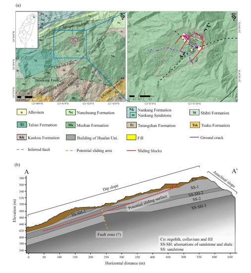
moves on the interface with a velocity of approximately 12 mm/year. The sliding surface is between the loosely consolidated colluvium and the underlying bedrock [29].
