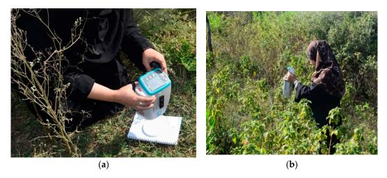
**Figure 3.** Data collection using the field spectroradiometer. Calibration using white reference panel avoiding shade (**a**); and taking the spectral reflectance of *Lantana camara* in the field (**b**).
