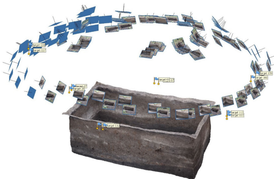
Figure 4. Example of the location of targets around a trench and the distribution of photographs taken to construct a model. The model depicted is that used for layer 6.
