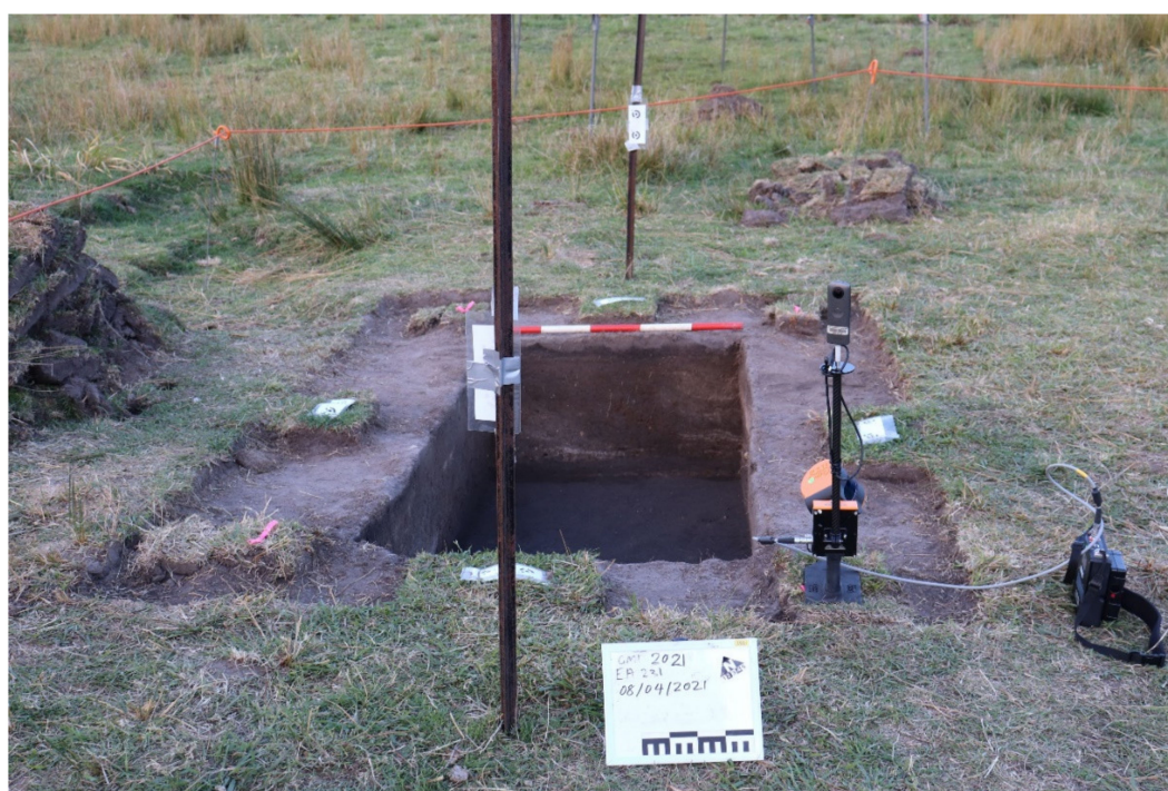
Figure 3. EA231 at the point of recording layer 6. An extra ca. 25 cm has been de-turfed to create a stable edge to the trench. PG targets are around the trench and on the Y fence posts. The GeoSLAM Zeb Horizon is located on one of the base points, with the others marked by pink flagging tape.
