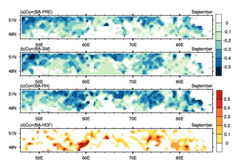
**Figure S4.** The spatial distribution of the correlation coefficient between burned area (a) precipitation (b) soil moisture (c) relative humidity and (d) hot days frequency in September over the Central Kazakhstan (CKZ) region. The linear trend of all variables is removed first before used for the calculation of correlation coefficient. The dots denote the regions where the correlation is statistically significant at the 90% confidence level.
