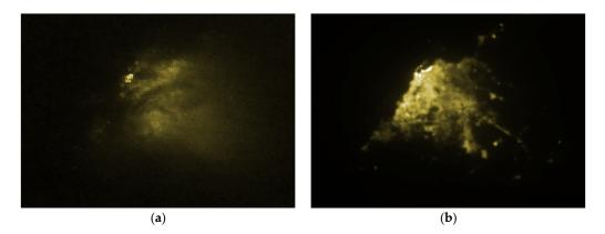
**Figure 2.** (a) Luanda city area in Angola is seen in unprocessed VIIRS night-time data acquired on 16 April 2020; (b) the image shows the same location in the processed VIIRS night-time data corrected for moon illumination and bad pixels using quality flags and then compositing for the entirety of April 2020.
