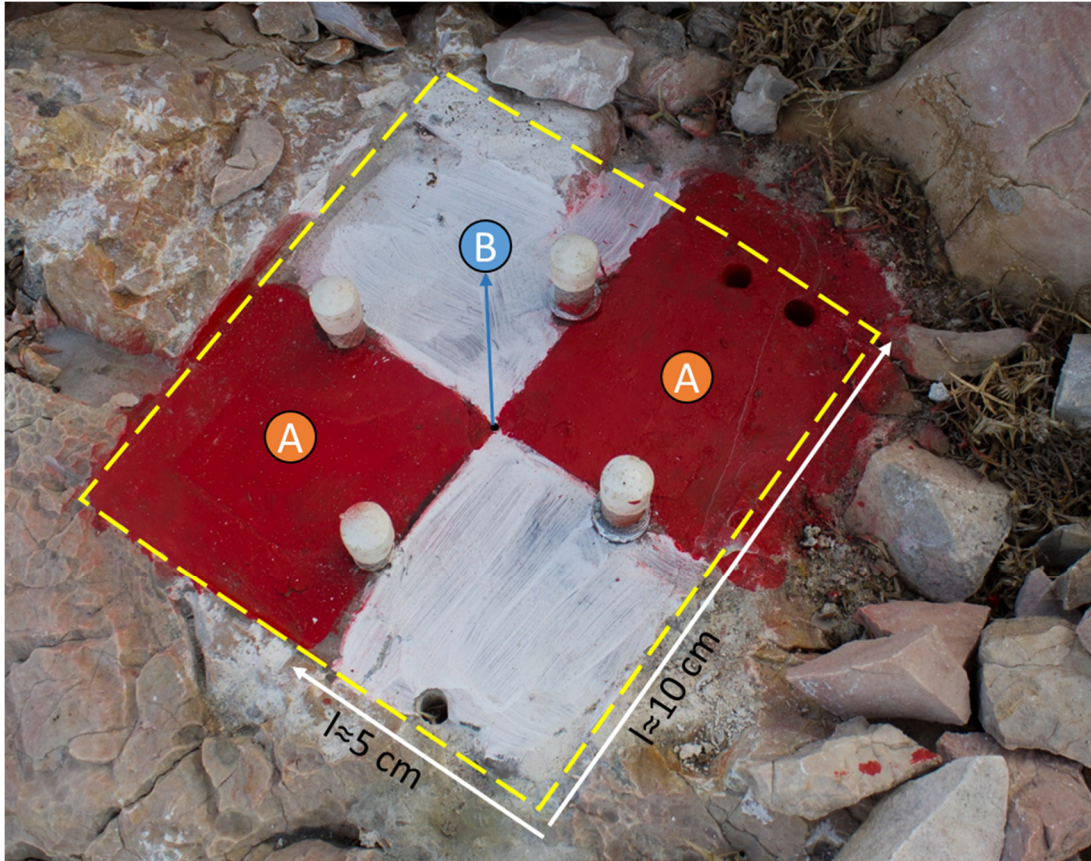
Scheme 1. Permanent GCP for repeat UAV photogrammetric surveys 1 2 .
