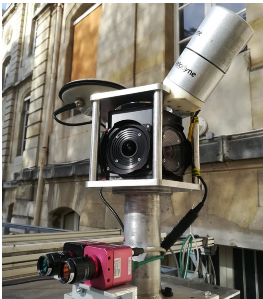
Figure 1. Prototype acquisition system used to create the PC3D dataset in the city of Paris. Sensors: Velodyne HDL32 LiDAR, Ladybug5 360° camera, Photonfocus MV1 16-band VIR and 25-band NIR hyperspectral cameras (hyperspectral data are not available in this dataset; they cannot be used in mobile mapping due to the limited exposure time).
