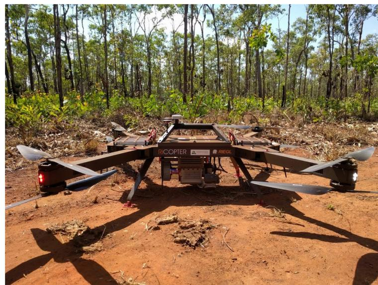
**Figure 2.** RIEGL RiCOPTER with VUX-1UAV.
