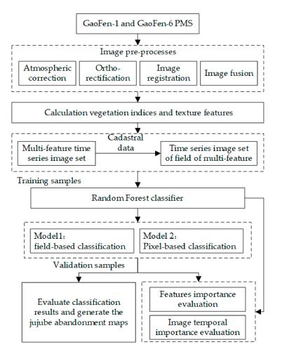
Figure 3. Flowchart of image processing.
