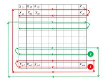
Figure 3. Visiting scheme of the SMMRF adopted in each layer of the first proposed method [18].
