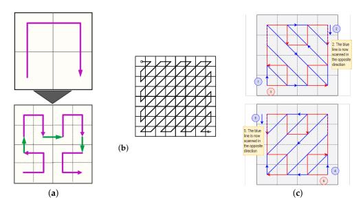
**Figure 4.** (a) Hilbert space-filling curve, (b) zig-zag scan, (c) symmetrized scan introduced for the second proposed algorithm through the combination of two Hilbert curve scans and four zig-zag paths.
