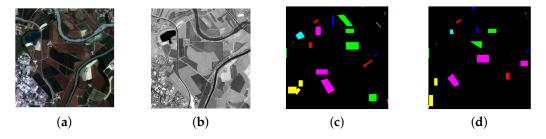
Figure 6. "Alessandria dataset": (a) RGB true-color composition of the IKONOS multispectral channels, (b) panchromatic channel, (c) training map, and (d) test map. Color legend for the classes: urban , agricultural , rangeland , bare soil , forest , water , wet soil .
