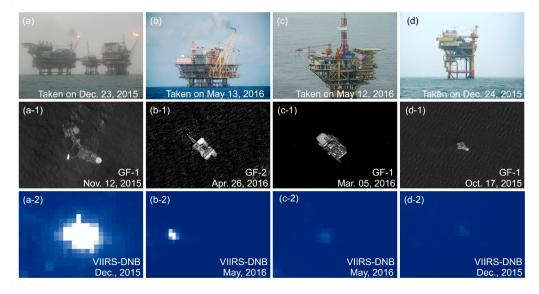
**Figure 2.** Image features of different HE targets: (**a**) is an oil platform group with gas flaring, (**b**) is a gas platform with gas flaring, (**c**) is a central processing platform without gas flaring, (**d**) is a wellhead platform without gas flaring; (**a**-1)–(**d**-1) are the corresponding panchromatic bands of high-resolution images; (**a**-2)–(**d**-2) are the corresponding NTL images.
