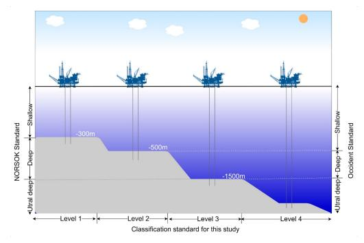
**Figure 7.** Depth classification for offshore HE in this study. Level 1:  $\geq$  -300 m, Level 2: -300 m > d  $\geq$  -500 m, Level 3: -500 m >d  $\geq$  -1500 m, d <- 1500 m.
