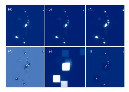
**Figure 4.** Data preprocessing: (a) original image; (b) negative adjustment image; (c) local Sigma filtered image, the window size is  $3 \times 3$ , Sigma factor is 4; (d) Hp image, convolution kernel is  $3 \times 3$ ; (e) Lp image, convolution kernel is  $27 \times 27$ ; (f) the difference between Hp image and Lp image. The parameters used in the above process are obtained through estimation and trial and error, and remain unchanged for all NTL images used.
