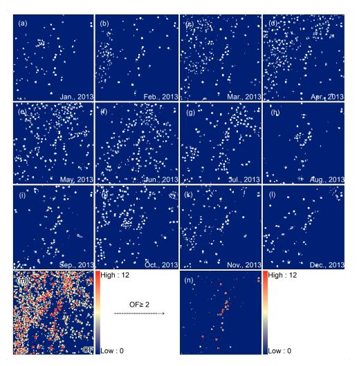
**Figure 5.** Target OF statistics: (**a**–l) are the binarized segmentation results of time-series images in one year, with a threshold t = 0.5; (**m**) is the OF statistics; (**n**) is the purified result, the threshold f = 2. The parameters used in the above process refer to empirical values, which are obtained through estimation and trial and error, and remain unchanged for all NTL images used.
