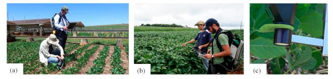
Figure 2. Spectral assessment in field (a,b) and detail of the plant probe device (c). Photo by Décio de Assis—Embrapa Soja.
