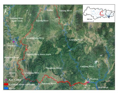
Figure 8. Critical river channels with higher flood risk.
