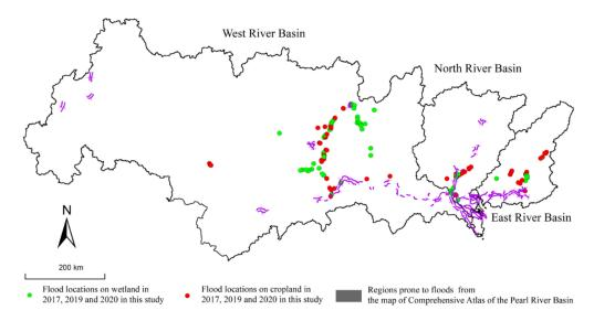
Figure 14. Comparison of the flood locations obtained in this study and the distribution of embankments obtained from the map of Comprehensive Atlas of the Pearl River Basin released by Pearl River Water Resources Commission (PRWRC) [52].
