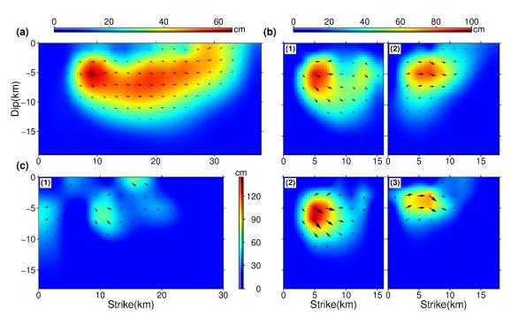
**Figure 4.** Slip distribution with arrows delineating the average rake of each sub-fault for the three test models, whose magnitude is color-coded. (**a**) Slip distribution for the optimal one-fault model. (**b**) Slip distribution for the optimal two-fault model, including the (1) northern fault and (2) southern fault. (**c**) Slip distribution for the optimal three-fault model, including the (1) secondary fault, (2) northern fault, and (3) southern fault.
