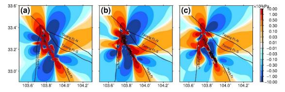
**Figure 9.** Static Coulomb stress changes on the 3D optimally oriented failure planes created by the Jiuzhaigou earthquake at different depths and the distribution of the aftershocks within 5 km. Coulomb stress changes at a depth of (**a**) 5 km, (**b**) 10 km, and (**c**) 15 km. Black dots represent the relocated aftershocks.
