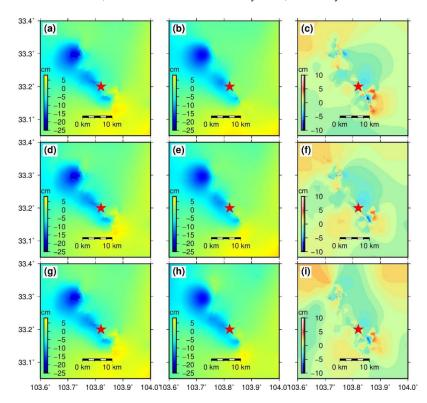
**Figure 3.** Comparison between interferometric synthetic aperture radar (InSAR) observations and predictions from the three test models. (**a**,**d**,**g**) Coseismic line-of-sight (LOS) deformation. Simulated LOS deformation from the (**b**) one-fault model, (**e**) two-fault model, and (**h**) three-fault model. (**c**,**f**,**i**) Residuals. Red star represents the epicenter of the 2017 Jiuzhaigou earthquake from the CEA-IGP.
