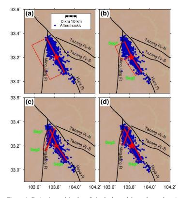
**Figure 2.** Projections of the four finite fault models on the surface, including the (**a**) one-fault model, (**b**) two-fault model (a northern fault and a southern fault), (**c**) three-fault model, and (**d**) brand-new two-fault model (a main fault and a secondary fault). Other symbols are the same as Figure 1b.
