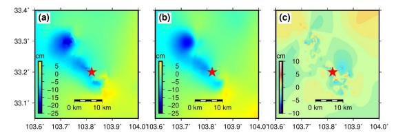
**Figure 6.** Comparison between InSAR observations and predictions from our preferred model. (a) Coseismic LOS deformation. (b) Simulated LOS deformation. (c) Residuals. Other symbols are the same as Figure 3.
