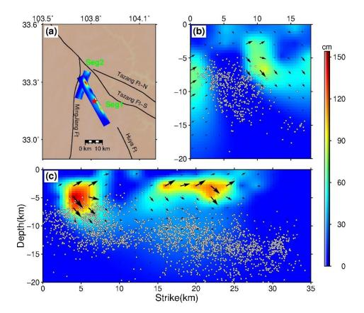
**Figure 7.** Slip distribution for our preferred model. (**a**) Projection of the slip model on the surface. Slip distribution of the (**b**) secondary fault, and (**c**) main fault. The white dots represent the relocated aftershocks. The slip distribution with arrows delineating the average rake of each sub-fault is color-coded. Other symbols are the same as Figure 1b.
