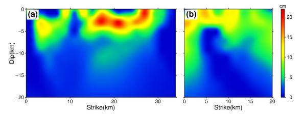
Figure 8. The standard deviations of the (a) main fault, and (b) secondary fault, based on the bootstrap method.
