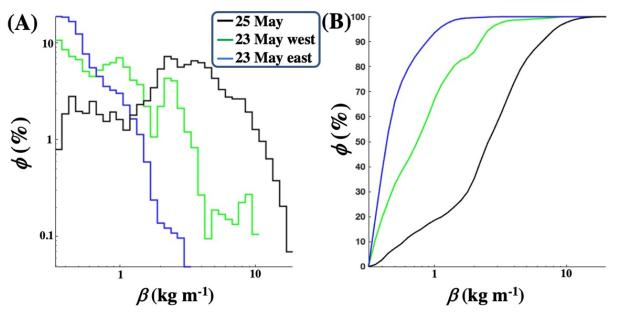
**Figure 13.** (**A**) Slick linear oil mass,  $\beta$ , (kg m<sup>-1</sup>) normalized probability distribution,  $\Phi$ , (normalized to kg m<sup>-1</sup> bin<sup>-1</sup>) for oil streamers from 23 May and 25 May. Data key on figure. See Figure 10A for the east and west slicks on 23 May. (**B**) Cumulative plot of  $\beta$ .
