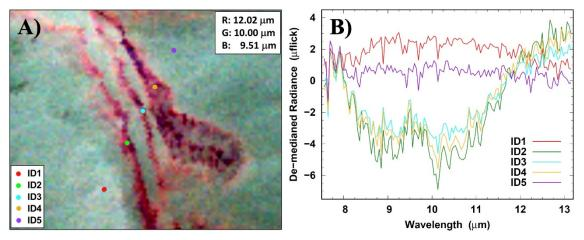
**Figure 3.** Spectral behavior of COP oil slick. (A) RGB coded radiance image with five spectral sampling locations shown. (B) De-medianed spectra extracted from sampling locations in panel (A).
