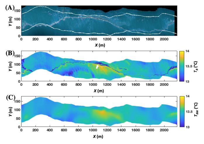
**Figure 6.** (A) Visible image photomosaic of an oil slick for 23 May in the along-slick and cross-slick coordinates, (X) and (Y), respectively. (B) Mosaicked thermal infrared image of sea surface brightness temperature ( $T_B$ ) projected to a 20-cm grid. The white arrow identifies the location of the image mosaic in Figure 7A. (C) Water brightness temperature,  $T_{BW}(X, Y)$ , respectively. Data key on figure.
