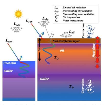
**Figure 1.** Oil slick thermal energy balance schematic illustrating the relationship between thickness, *h*, and oil-water thermal contrast.
