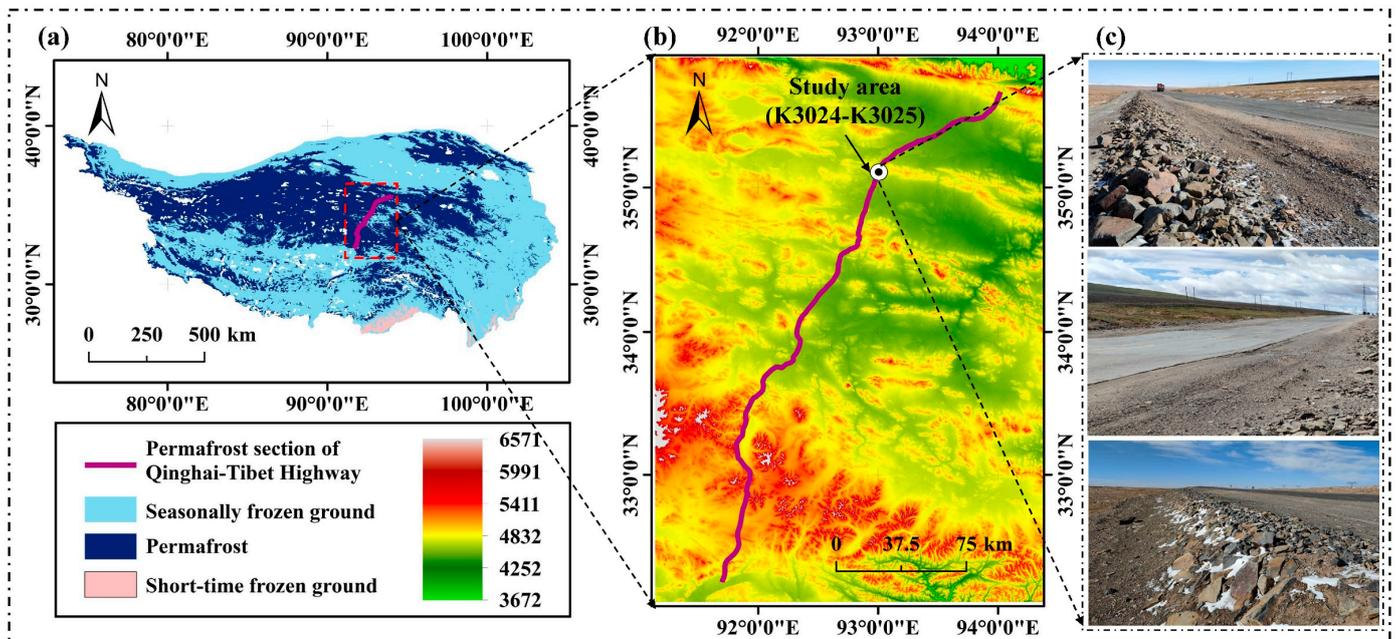
**Figure 2.** Study area: (a) spatial distribution of permafrost region in the QTP (the permafrost map is from [61,62]); (b) the location of k3024 to K3025 in the QTH; (c) field photographs of k3024 to k3025, from top to bottom: “wavy” pavement; local settlement of embankment and the block-stone embankment.
