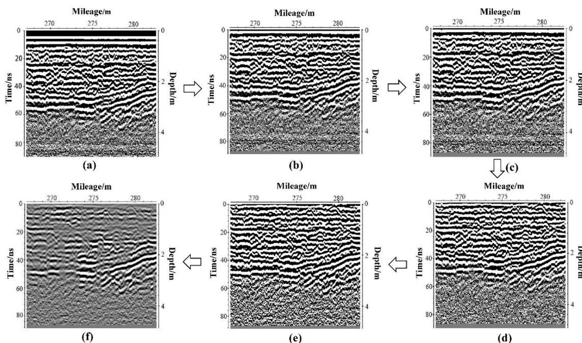
**Figure 7.** GPR data processing flow: (a) input data; (b) remove direct waves; (c) exponential gain; (d) average path extraction; (e) 1-D filtering; (f) 2-D filtering.
