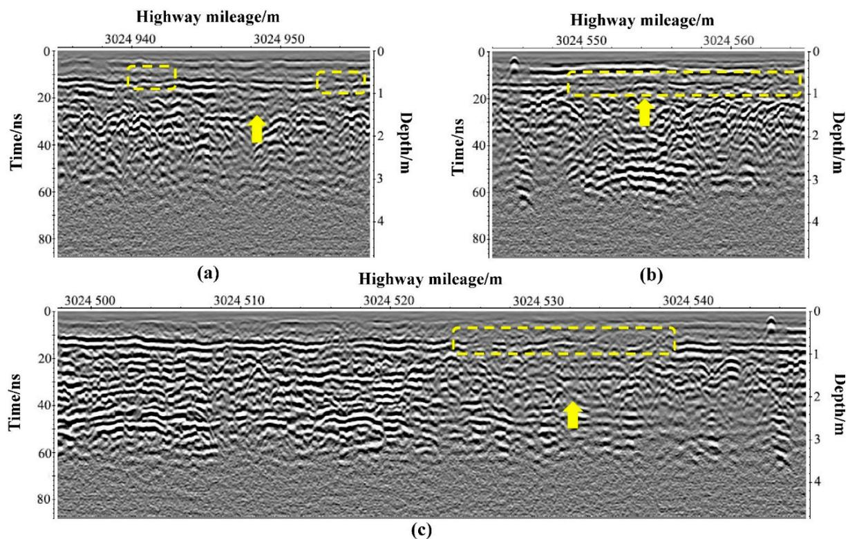
**Figure 8.** GPR images of the loosening of the upper sand-gravel layers: (a) K3024 + 935 to K3024 + 956; (b) K3024 + 544 to K3024 + 565; and (c) K3024 + 498 to K3024 + 548. The yellow dashed box shows the abnormal area of the sand-gravel layer, and the yellow arrow is used to facilitate reading.
