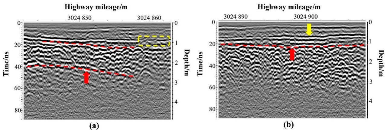
**Figure 10.** GPR images indicating the settlement of the block-stone layer: (a) K3024 + 842 to K3024 + 863; (b) K3024 + 887 to K3024 + 909. The yellow dashed box shows the abnormal area of the sand-gravel layer, the red dotted line indicates the settlement trend of the block-stone layer, and the yellow and red arrow is used to facilitate reading.
