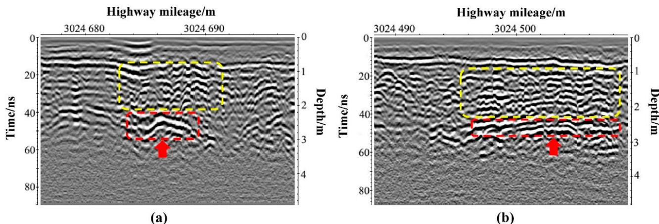
**Figure 9.** GPR images indicating looseness of the block-stone layers: (a) K3024 + 676 to K3024 + 697; (b) K3024 + 488 to K3024 + 509. The yellow dashed box shows the abnormal area of the block-stone layer, the red dashed box shows the abnormal area of the ground, and the yellow and red arrow is used to facilitate reading.
