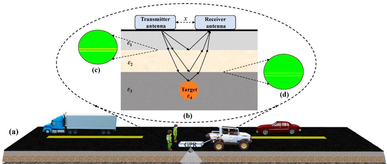
**Figure 5.** Schematic diagram of the GPR survey on the highway: (a) highway; (b) the electromagnetic waves emitted by the transmitting antenna are reflected by the different layers and then return to the receiving antenna; (c) strong electromagnetic wave reflection; (d) weak electromagnetic wave reflection.
