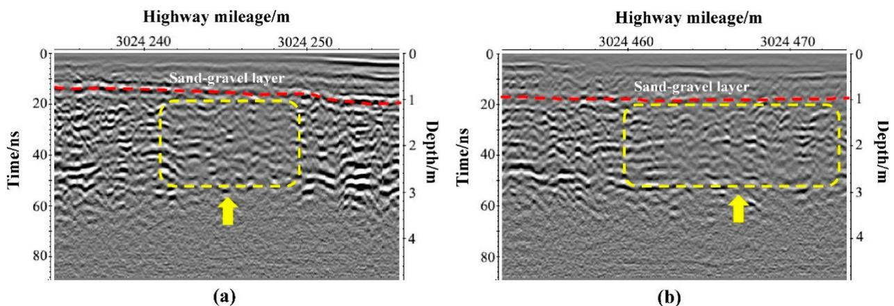
**Figure 11.** GPR images of an abnormally dense block-stone layer: (a) K 3024 + 235 to K3024 + 256; (b) K 3024 + 452 to K3024 + 474. The yellow dashed box shows the abnormal area of the block-stone layer, the red dotted line indicates the boundary between the sand-gravel layer and the block-stone layer, and the yellow arrow is used to facilitate reading.
