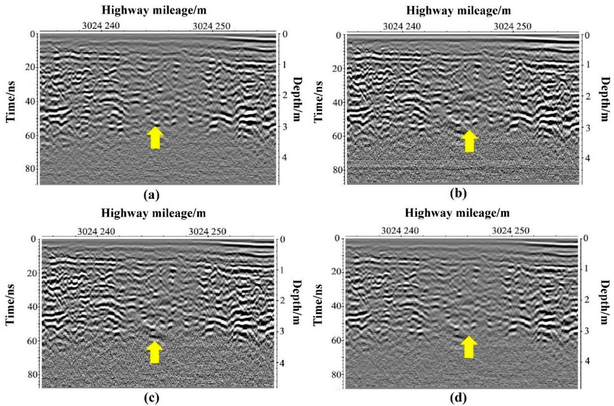
**Figure 12.** Comparison of the results of different processing methods for abnormally dense areas: (a) processed according to the normal flow; (b) after direct wave removal only gain processing was performed; (c) only horizontal signals were removed based on the previous step; (d) only moving-average processing was performed based on the previous step. The yellow arrow is used to increase visibility.
