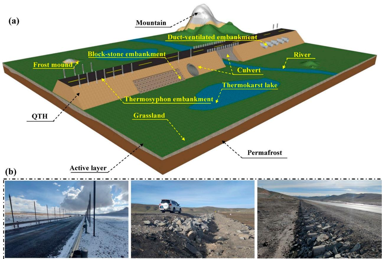
**Figure 1.** (a) Proactive temperature-controlling measures and the surrounding environment along the QTH; (b) field photographs, from left to right: thermosyphon embankment; block-stone embankment, and duct-ventilated embankment.
