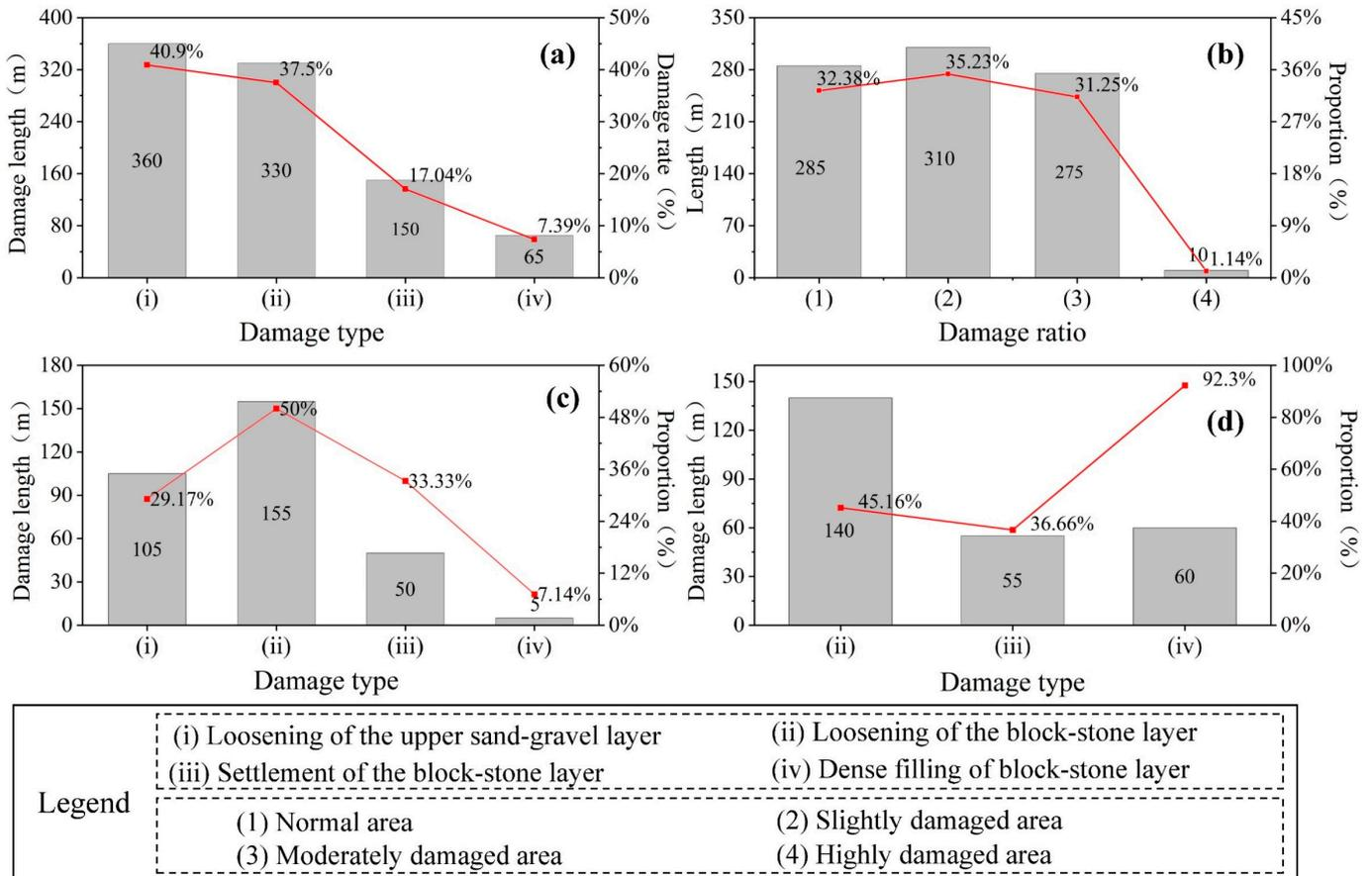
**Figure 14.** Relationship of different types of damage in the block-stone embankment: (a) shows the damaged length and rate of the different types of damage; (b) shows the length and proportion of highway sections with different degrees of damage; (c) shows the relationship between the different types of damage and the abnormality of the lower part of the embankment; (d) shows the relationship between the different types of damage and the loosening of the upper sand-gravel layer.
