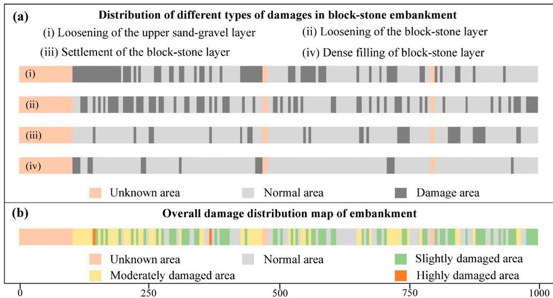
**Figure 13.** For the K3024 to K3025 section: (a) distribution of different types of damage in the block-stone embankment. Note: the unit (five meters as a unit) was considered damaged if the unit was damaged more than half, otherwise, it was a normal unit. (b) overall damage situation of the embankment. Note: The degree of embankment damage was based on the number of damaged species on each unit.
