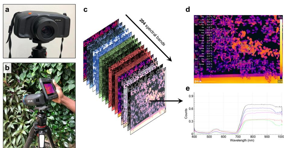
**Figure 5.** (a) the SpecimIQ hyperspectral camera and (b) the FLIR T560 thermal camera used to monitor the indoor VGW. (c) Illustration of multiband acquisition of the spectral images from the SpecimIQ data (204 bands in the range of 400–1000 nanometer) and (d) a thermal image of the wall acquired from the FLIR T560 camera. (e) Spectral signal of specific pixels from the VGW image. Images (a,b) were taken by D. Helman.
