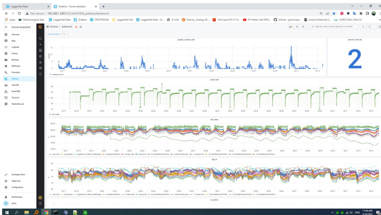
**Figure 3.** Screenshot of the Grafana interactive visualization web application (<https://grafana.com>; accessed on 1 June 2022), showing from top to bottom real-time data of the number of persons (blue), the water level at the tank (green), temperature, and RH conditions from the sensors inside the workplace.
