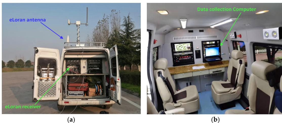
**Figure 11.** Test platform for cycle identification method: (a) outside of the test platform; (b) inside of the test platform.
