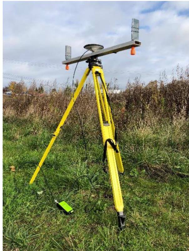
Figure 1. Test area with experiment on Huawei P30 Pro static DGPS positioning accuracy.
